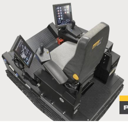
Touch enabled Operator Consoles with functional Status, Permissive and Control screens.
